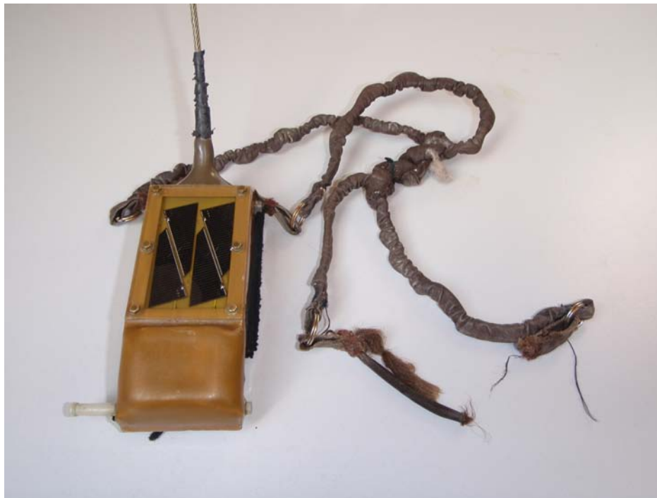
Fig. 7. Satellite-transmitter bitten off by Greylag Goose in the Netherlands.
